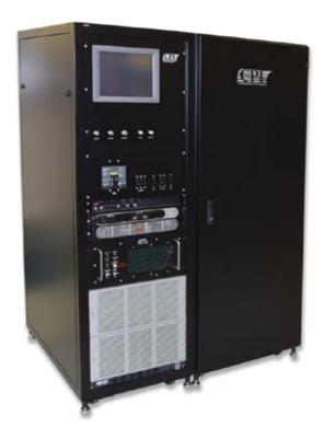
The CPI BMD 250 kW, C-band, klystron transmitter components for weather radar are available for constructing a complete microwave transmitter. This microwave transmitter uses a CPI klystron amplifier (VKC8387) as the final RF output device. CPI is able to furnish a compact, user-friendly, cost-effective microwave power source with excellent pulsed Doppler capability.
